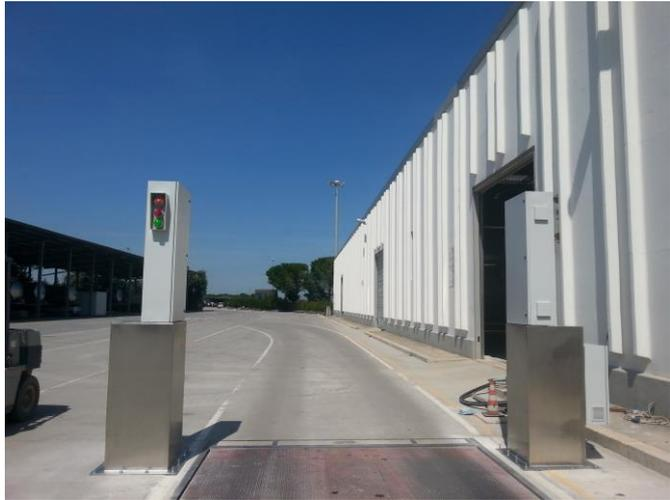
Example of the Portal Monitor with the scintillation detectors
